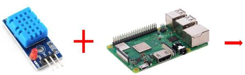
The DHT11 is a basic, ultra low-cost digital temperature and humidity sensor. It uses a capacitive humidity sensor and a thermistor to measure the surrounding air, and spits out a digital signal on the data pin (no analog input pins needed). Its fairly simple to use, but requires careful timing to grab data.
