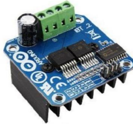
Model: BTS7960 Current rating: Max 43 Amp Voltage: 24 V
